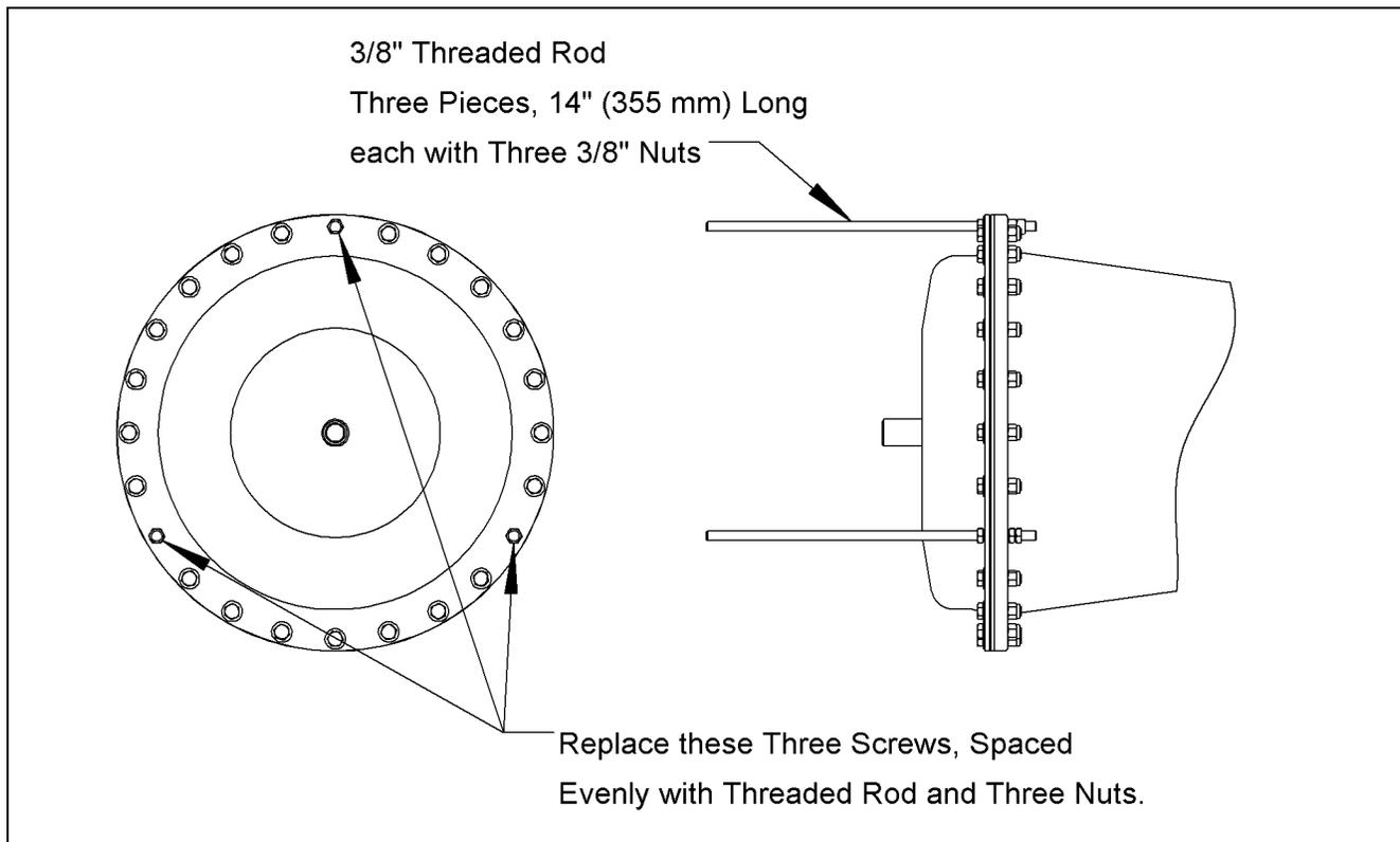
**Figure 3 - Stud Requirements for Diaphragm Cover Removal**
