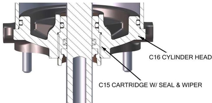
7. Remove Cylinder Cartridge (C15). Use a spanner wrench to unscrew the Cylinder Cartridge (C15) out of the Cylinder Head (C16). See Figure 5.
