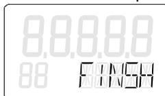
In the first line, the determined stroke in mm will appear in additional if the set lever length has been entered with the parameter 3.YWAY.
