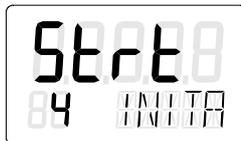
During the initialization process "RUN1" to "RUN5" appear one after the other in the lower display.
