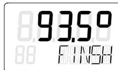
The upper value shows the total angle of rotation of the actuator (example 93,5°).
