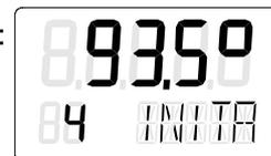
To exit **Configuration** mode press the mode key
