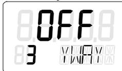
You only have to set this parameter if you want to have the calculated total stroke displayed in mm at the end of the initialization phase. To do that, select the same value in the display as the value to which you set the driver pin on the scale of the lever.
