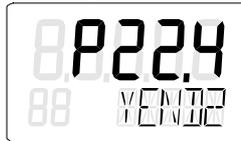
Now drive the actuator with the increment (+) and decrement (-) keys to the position that you wish to define as the second end position. Then press the mode key
