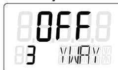
This parameter only has to be set if you wish to have the determined total stroke displayed in mm at the end of the initialization phase. To do this, select the same value in the display that you have set with the driver pin on the lever scale, or the next highest value for intermediate settings.
