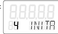
To exit **Configuration** mode press the mode key
