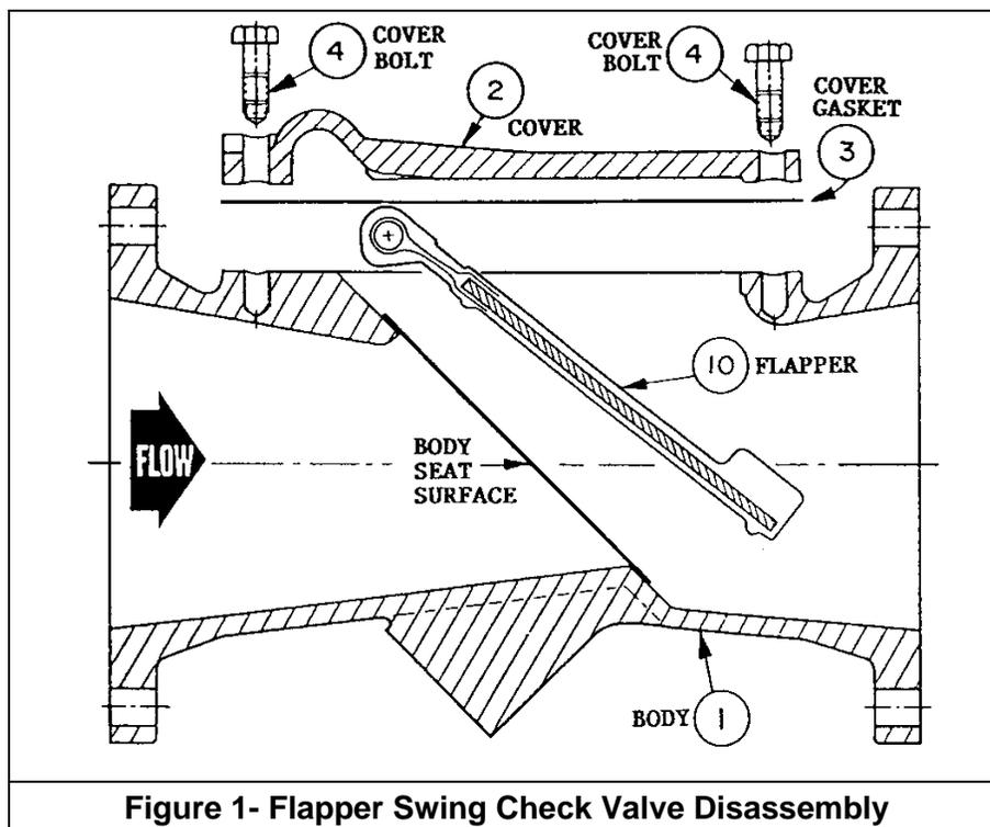
5. To reassemble, replace Cover Gasket (3), often the same cover gasket can be reused several times.
